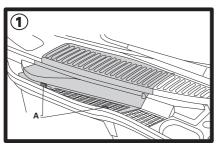
Release clips (A) by pulling towards front of vehicle, raise the cover and lift it out.
