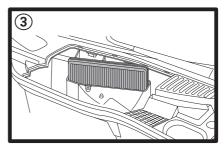
Remove used filter noting flow direction, replace with new Ryco RCA144P.
